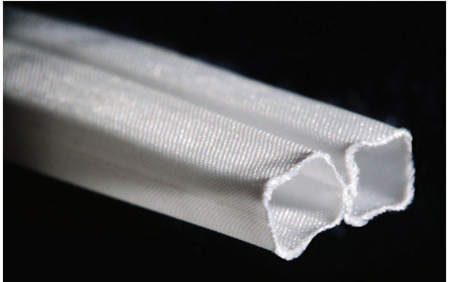
Expertise in material selection and textile forming technologies yields structures such as these biluminal, woven polyethylene terephthalate (PET) tubes.
