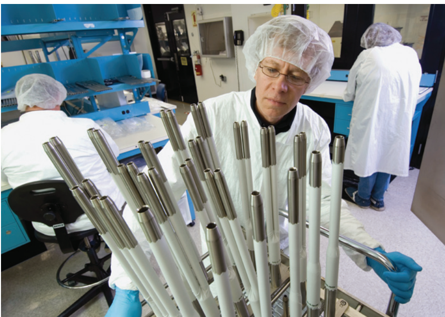
A Secant Medical textile specialist performs an inspection prior to processing bifurcated graft structures used in the treatment of abdominal aortic aneurysms.
